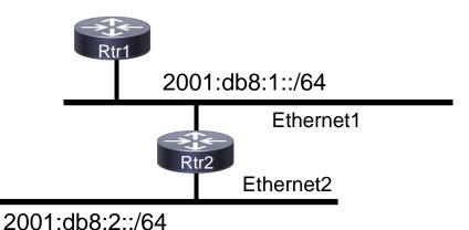
Redistributing both IPv6 static routes and IPv4 static routes.
